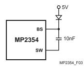
Figure 3—External Bootstrap Diode
