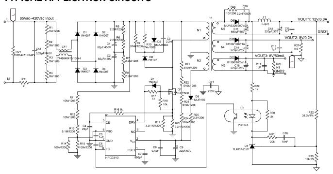
**Figure 6: Typical Application Schematic**
