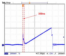
Figure 5: Leading-Edge Blanking
