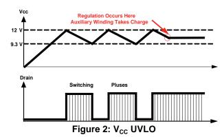
The lower threshold of VCC under-voltage lock-out (UVLO) decreases from 9.3V to 6.2V when fault conditions occur, such as OLP, OVP, and OTP.
