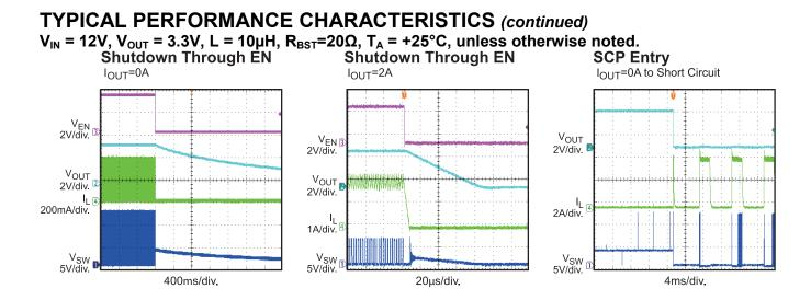
SCP Entry I<sub>OUT</sub>=2A to Short Circuit
