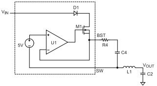
Figure 3: Internal Bootstrap Charging Circuit
