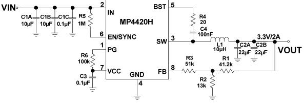
Figure 8: 3.3V Output Typical Application Circuit
